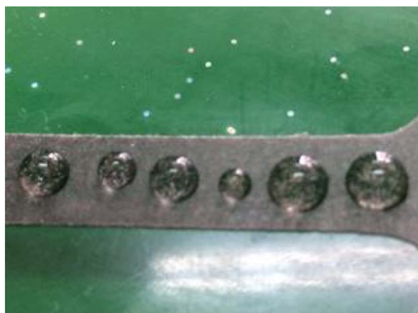
Figure 6. Water droplets sitting on the composite film. [Color figure can be viewed in the online issue, which is available at wileyonlinelibrary.com.]
